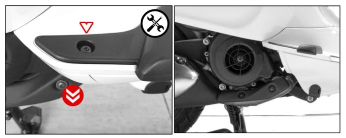
Unscrew the flange connection of the serial header, loosen the brackets screws and remove the stock exhaust.
