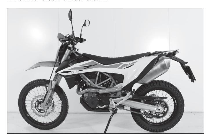
Remove the seat and the front side covering. In the next step remove the rear side covering.
