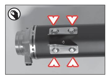
Remove the stock bracket and mount it onto the REMUS sport exhaust.
