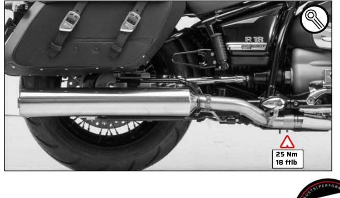
Mount the heat shield from the stock exhausts onto the REMUS sport exhausts.
