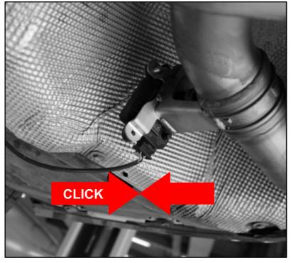
Connect both actuators with the REMUS actuator cable.
