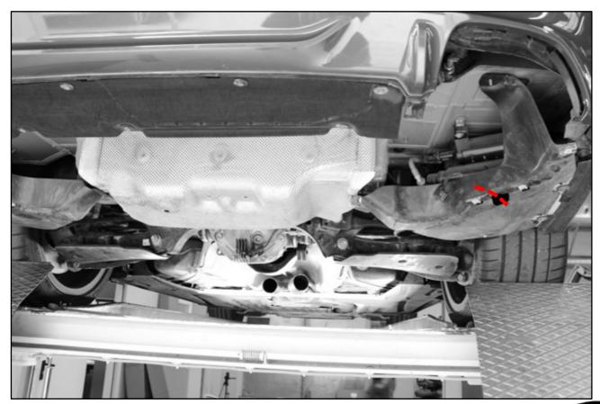
Connect the supplied REMUS actuator cable and guide the cable behind the heat protection shield all the way to the other side.
