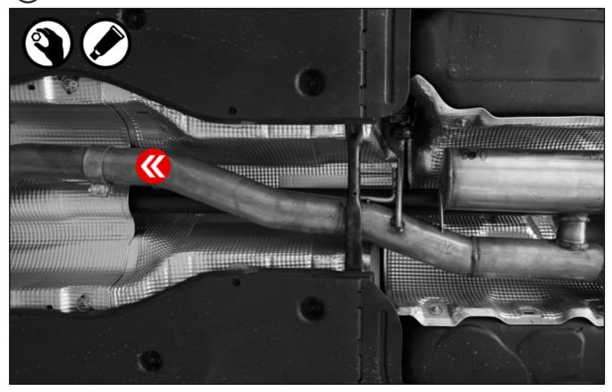
Mount the bracket onto the rubber hanger.
