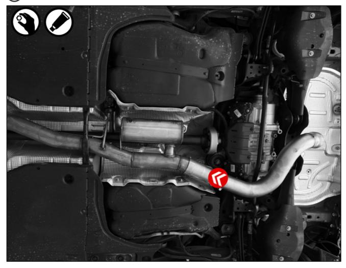
Mount the bracket onto the rubber hanger.
