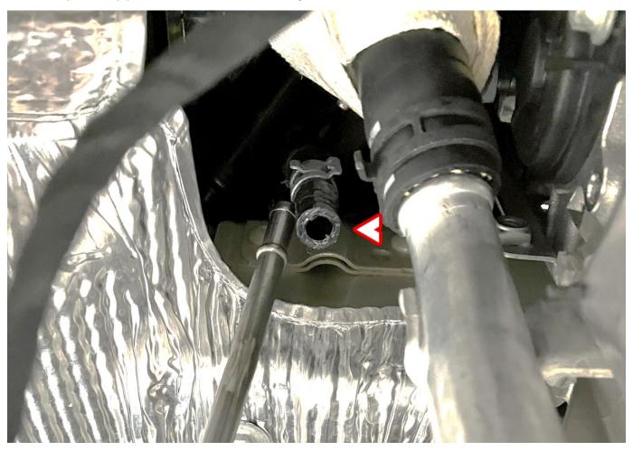
Reposition the hose clamps and secure the pressure pipe with them.
