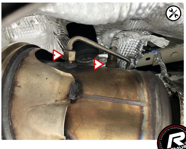
Loosen the highlighted screws on the right-hand side.
