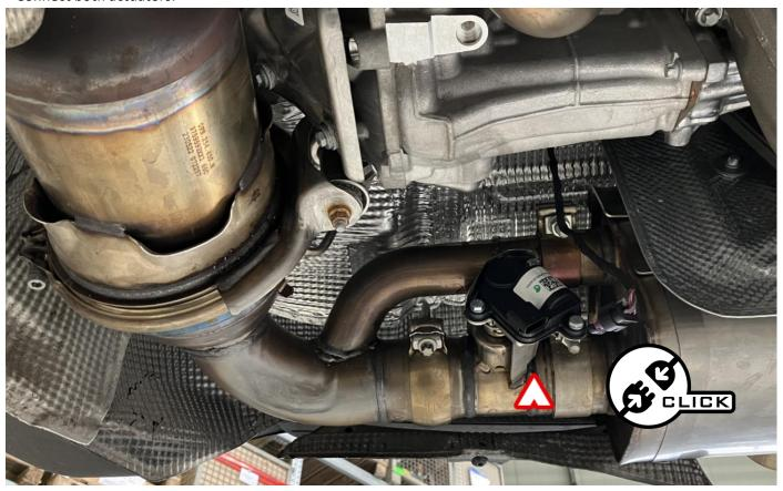
Turn both valve tubes upwards to ensure sufficient clearance to other components.
