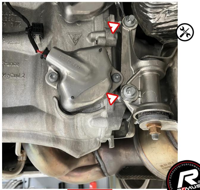
Loosen the highlighted screws on the left-hand side.
