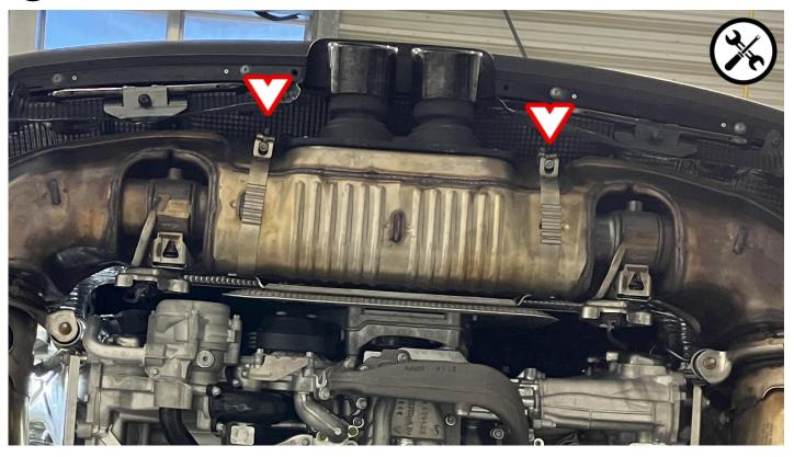
Loosen the clamps of the catalytic converter and take them off.
