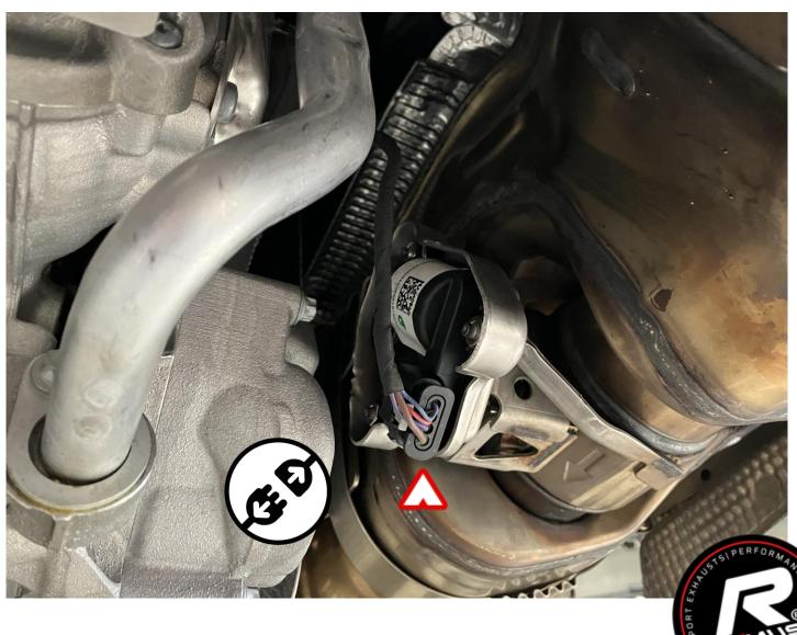
Detach the pressure hose on the left and right side. Remove the highlighted screw.
