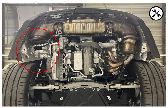
Next, remove the right catalytic converter.
