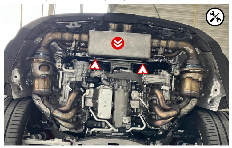
Install the tubes by using V-band clamps of the stock exhaust system.
