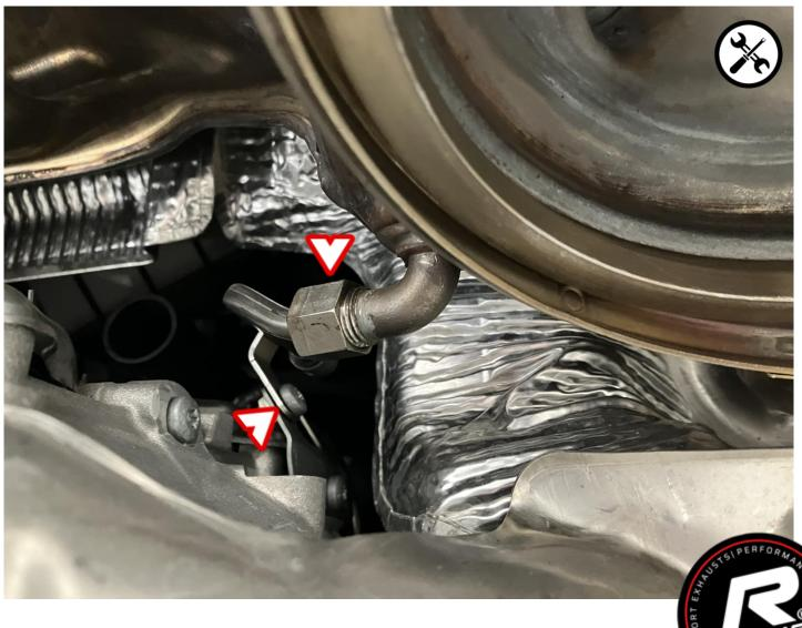
Dismount the pressure hoses and O2 sensors from the catalytic converters.
