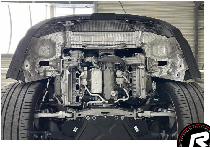
Remove the pressure hoses on the left and right by squeezing the hose clamps together and sliding them upwards.
