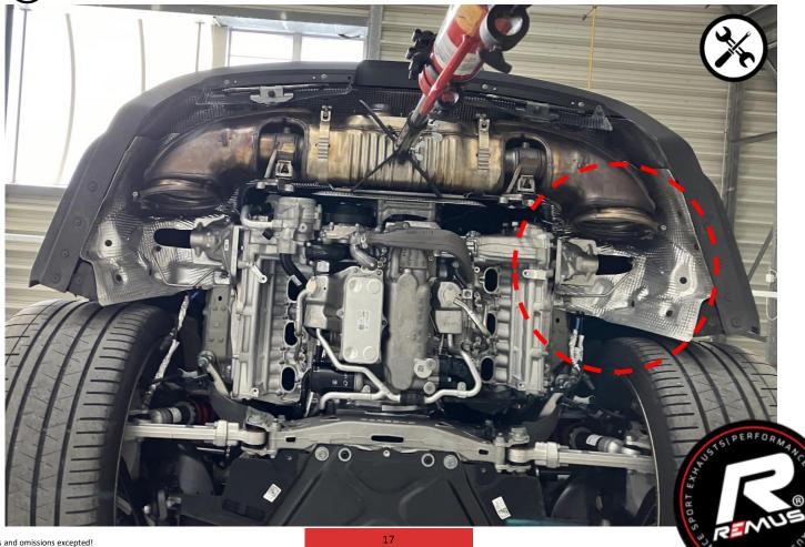
Unhook both exhaust clamps and remove the rear silencer.
