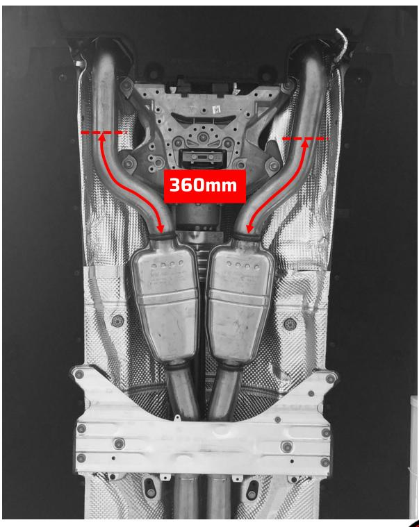
Mount the REMUS front silencer replacement tubes onto the stock pipes.
