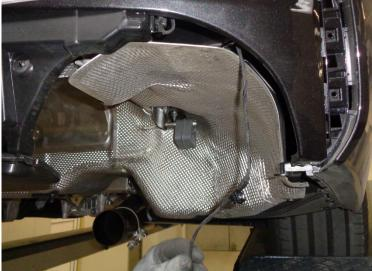
Guide the actuator cable underneath the heart shield and fix it onto the heat shield by using the clip.
