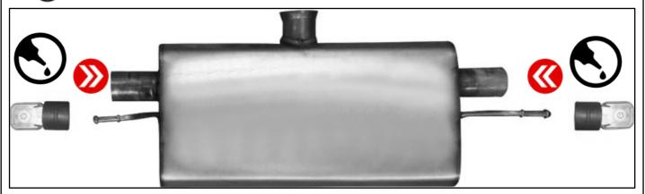
Install the REMUS connection tube on the original tube, if necessary use the supplied adapter.
