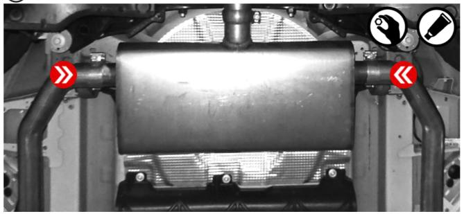
Align the exhaust system and tighten all connections.
