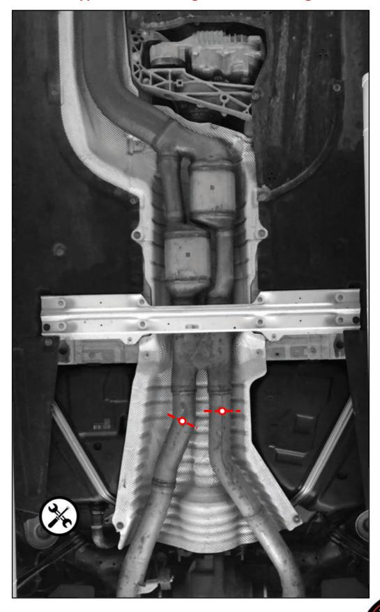
Unhook and unscrew the rubber hangers, unplug the actuator and remove the stock exhaust system.
